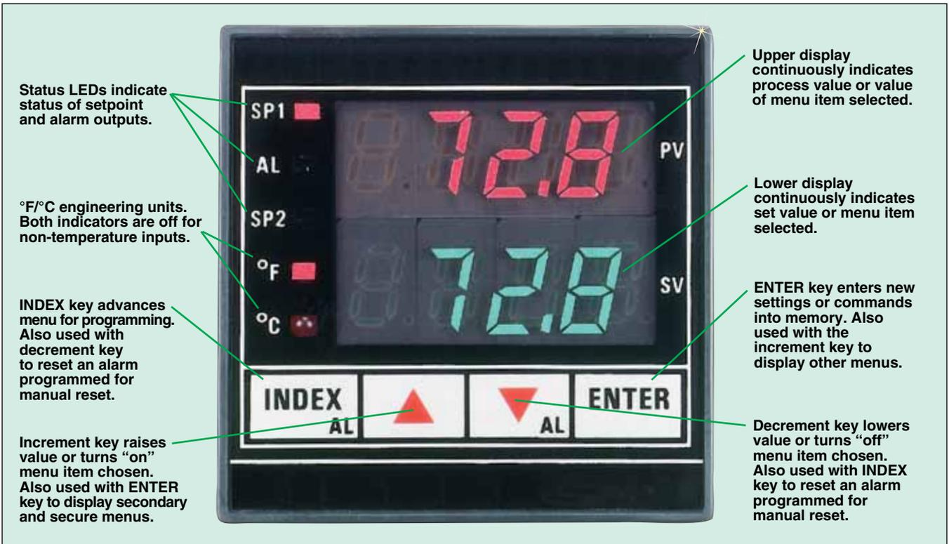
The CN76000 1/6 DIN controllers provide economical control for a wide variety of processes, including heating, cooling, and heat/cool. When used with the proper transmitters, these devices can also control pressure, flow, humidity, motion, or pH. The front panel is NEMA 2, 3R, and 12 rated for waterproof protection and is corrosion resistant.
